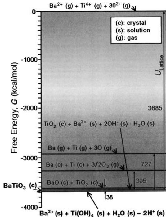
Figure 2 Energy diagram for the formation of BaTiO<sub>3</sub> at 25°C. Huge excess of energy is necessary to create, vapor, gas or ion (plasma) from the solid as compared to creation of aqueous solution at the same temperature. This gives the thermodynamic explanation why processing of the advanced materials using aqueous solution consumes low energy in contrast to vapor/plasma processing.
