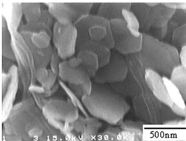
Figure 9 LiCoO<sub>2</sub> films composed of nano- powders fabricated on PTFE membrane by electrochemically activated interfacial reaction methods at 1mA/cm<sub>2</sub> in 0.1M CoSO<sub>4</sub> and 5M LiOH at 120°C for 30 min [46].
