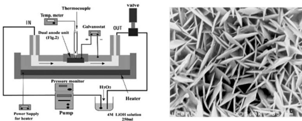
Figure 8 (a) Schematics of the flow-cell system for hydrothermal-electrochemical reactions, (b) LiCoO<sub>2</sub> film on a Pt substrate prepared in the flow-cell system at 150°C for 2 h with 1mA/cm<sup>2</sup> current [40].
