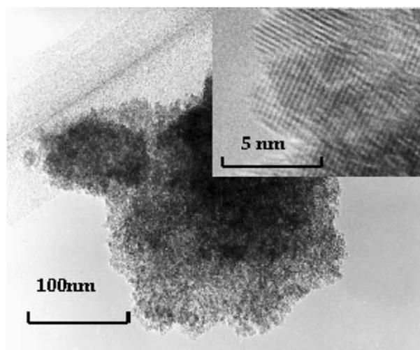
Figure 5 Zr<sub>0.6</sub>Ce<sub>0.4</sub>O<sub>2</sub> nano-crystals by Hydrothermal method with ball milling at 120°C for 6 h, 100 nm size powders consist of about 6 nm crystals [15].
