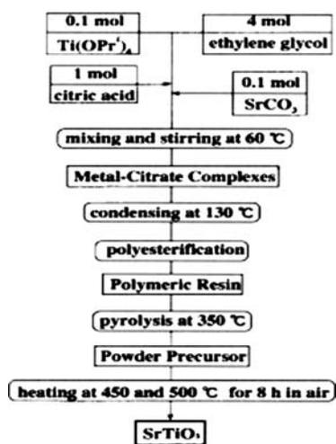
Figure 3 Flow chart for preparing SrTiO<sub>3</sub> by the Polymerized Complex Method. The molar ratio of Ti(OPr)<sub>4</sub>/SrCO<sub>3</sub>/CA/EG = 0.1/0.1/1/4 [6].
