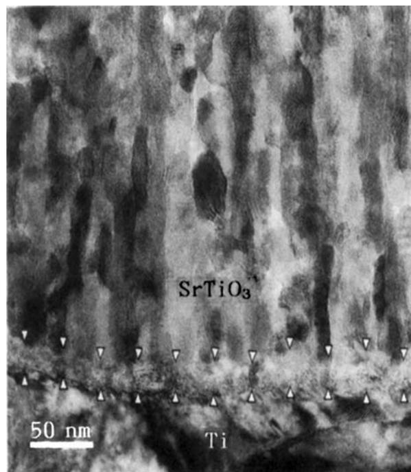
Figure 6 Magnified TEM Image of the  $SrTiO_3$  film/Ti substrate interface of the  $SrTiO_3$  film with potentiostatic electrolysis at +8.0 V vs. Ag/AgCl in 0.5M  $Sr(OH)_2$  Solution of pH 14.2 at  $150^\circ\text{C}$ . Arrows indicate boundaries of a polycrystalline layer of Ti oxides whose microstructure is different from the columnar one of the overlying, inner  $SrTiO_3$  layer [30].
