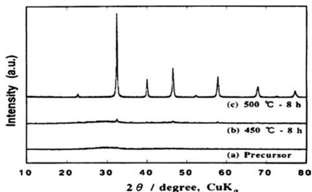
Figure 4 X-Ray diffraction patterns of the Polymerized Complex-derived Powder precursor for SrTiO<sub>3</sub> (a) and of samples heat-treated in static air at 450°C for 8 h (b) and 500°C for 8 h (c) [6].
