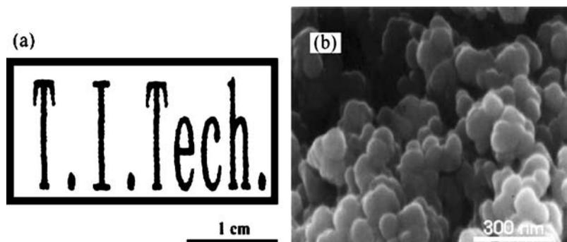
Figure 10 (a) Photograph of a PbS pattern on a paper prepared by the ink jet reaction from aqueous solutions at a room temperature. (b) SEM photograph of the same sample. The pattern consists of consolidated PbS crystals with 50-100 nm size [47].
