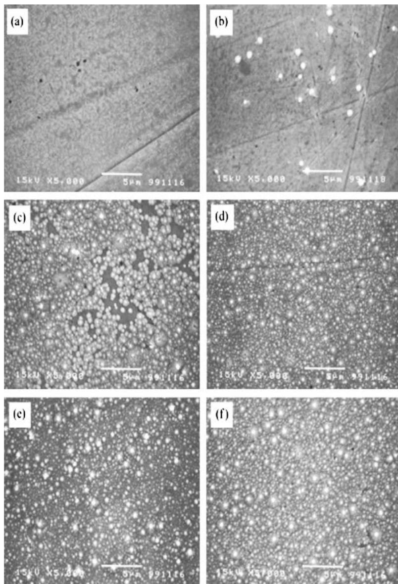
Figure 7 BaTiO<sub>3</sub> film formation on a Ti substrate by microwave-hydrothermal method in Ba(OH)<sub>2</sub> solution at 100°C, (a) Ti substrate, (b) 5 min, (c) 10 min, (d) 15 min, (e) 30 min, and (f) 60 min. [44].
